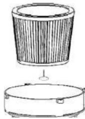
Clean the areas covered by the filter and insert a new filter by following the removal procedure above in the opposite order.
