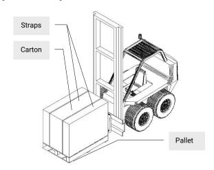
To unpack the machine, cut the straps that secure the carton to the pallet and then remove it. Once unpacked, the machine can be lifted by running the hoisting slings through the hooks provided. Below are some safety instructions for transport and handling operations.
