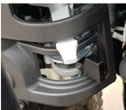
Fig4: Warm start or trouble start position - Engine Fuel tap lever (black) to the right and choke lever (grey) in centre position. Don't forget to move this choke lever immediately to the right (off position) when the engine starts running
