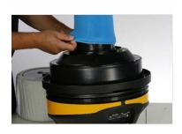
Ensure the head is correctly fitted and the clips secure. For dry, non- hazardous material, ensure the HEPA filter is fitted.
