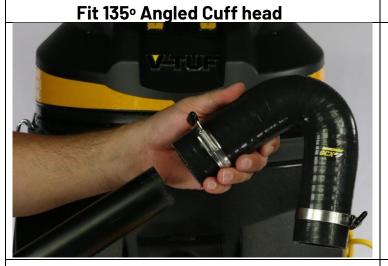
Tighten Thumb Screw 2(Nm).
