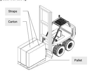
To unpack the machine, cut the straps that secure the carton to the pallet and then remove it. Once unpacked, the machine can be lifted by running the hoisting slings through the hooks provided. Below are some safety instructions for transport and handling operations.
