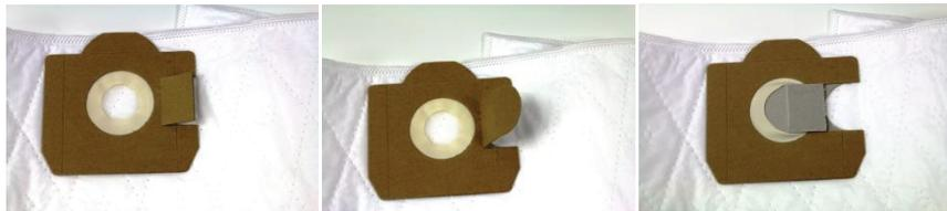
Fit the new filter bag, making sure that the bag's membrane seal fits perfectly over the internal slot of the tank inlet and that the bag fits neatly around the edge of the tank internal. Refit the head ensuring that the clips are completely closed and there is no parts of the dust bag exposed.
