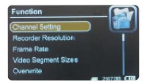
1. Channel Setting: Press 🖺 / 🏞 to select "Channel Setting", and then press 🗖 to enter
