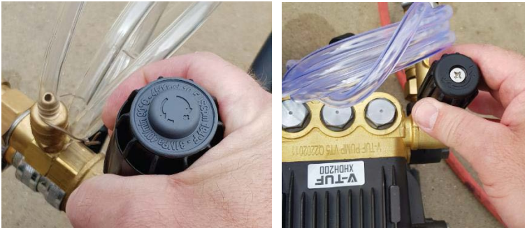
Fig1: Pressure adjustment knob (these may differ in looks) – turn anticlockwise (to low pressure) for starting. This will make it easier to start and also reduce unnecessary wear on your engine pull start mechanism.
