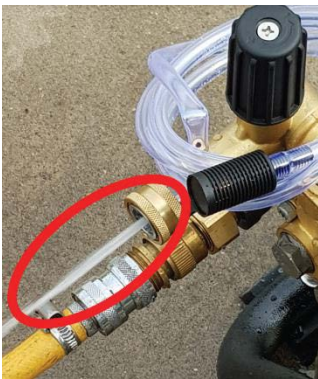
Fig2: High pressure outlet: This is where the high-pressure hose connects. The image shows the high-pressure hose disconnected and a jet of water jetting out. This is normally done when priming (getting the air out and water in) the pump when the machine is used on suction. Run the engine until you get a strong stream of water jetting out, then stop the engine and connect the high-pressure hose, then restart with the pressure adjustment knob set on low pressure.
