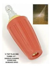
**V-TUF T3.26 turbo nozzle** creates a straight pencil jet which is spun to create a conical shaped water jet. This makes the turbo nozzle extremely useful and efficient when it is used for cleaning surfaces.
