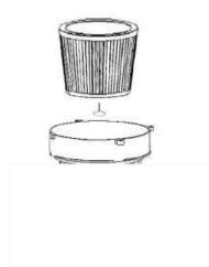
Clean the areas covered by the filter and insert a new filter by following the removal procedure above in the opposite order.
