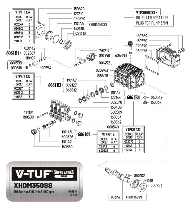
LUBRICATION OF THE PUMP We recommend: VTUF PL100 – OIL CAPACITY 0.42 kg You should change the oil after the first 50 hours of use, and after each subsequent 500 hours of operation.
