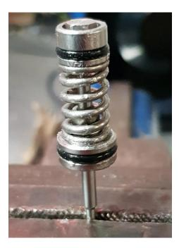
4. To adjust the length, hold the spindle in the vice, as shown and rotate the hex head clockwise to shorten the spring and anticlockwise to lengthen.
