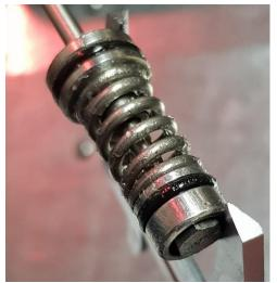
1. Hold the callipers with the measuring one measuring edge on the flat surface of the collar around the hex head. Please note: NOT on the hex head.
