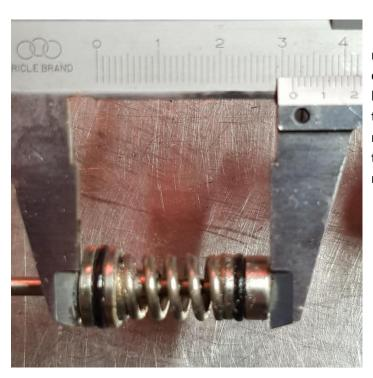
3. Please note: this measurement must be no less than 31.7mm. This will overload the machine and cause fuse blowing. If this measurement is longer the pressure will be lower on the machine. Use thread locker on the thread on this mechanism so this measurement is maintained.
